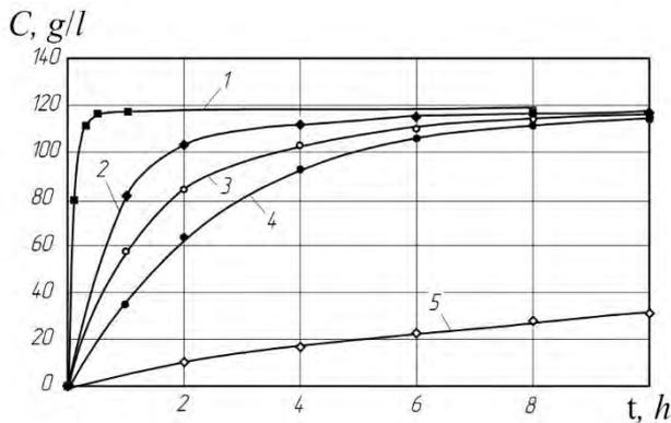
Fig. 1. Kinetics of oil extraction for not grinded and grinded sunflower seeds of different fractions with *n*-hexane at the boiling temperature of the solvent in the apparatus with a mixer: 1 – grinded seeds with  $d_{mid} = 0.3$  mm; 2 – grinded seeds with  $d_{mid} = 0.5$  mm; 3 – grinded seeds with  $d_{mid} = 0.75$  mm; 4 – grinded seeds with  $d_{mid} = 1.25$  mm; 5 – not grinded seeds
