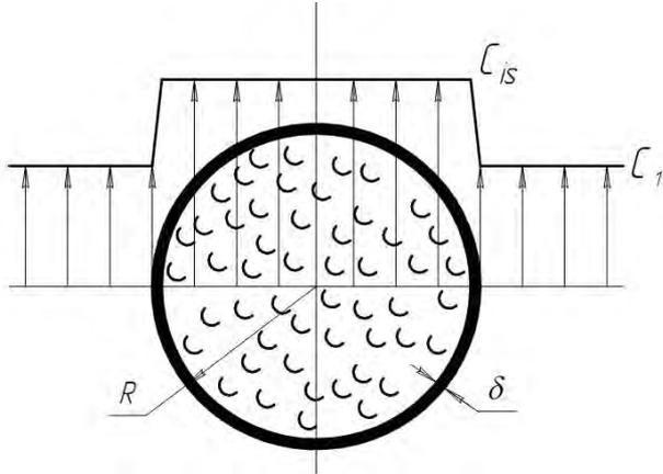
Fig. 3. Scheme of a simplified physical model of extraction of target components from sunflower seeds ( $\delta$  – film thickness,  $C_1$  – the concentration of oil in the main mass of solution,  $\text{kg/m}^3$ ;  $C_{is}$  – the initial concentration of oil in the seed,  $\text{kg/m}^3$ )
