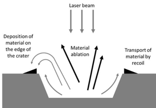
Fig. 1. Scheme of the laser beam operation
