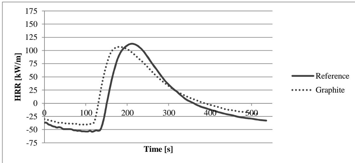
Fig. 4. Heat release rate from cone calorimetry for reference and containing graphite ceramizable composites
