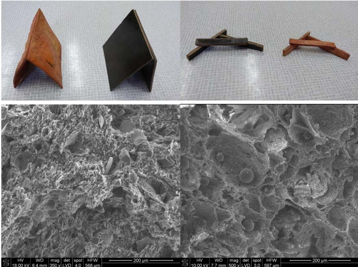
*Fig. 2. The higher photographs show how is changing the structure of ceramizable composites macroscopically (darker samples - before ceramization, lighter samples - after ceramization). The lower photos from the scanning electron microscope illustrating how the micro-morphology of the ceramizable composites changes (on the left before ceramization, on the right after ceramization).*
