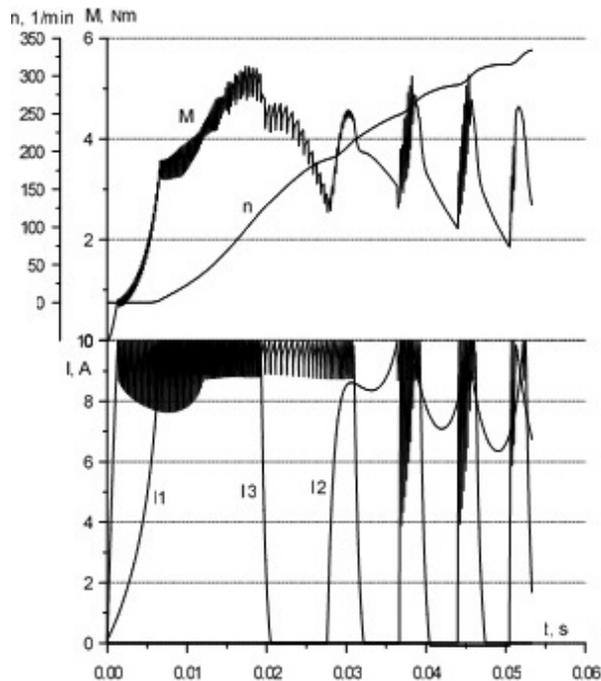
Fig. 4. Start transient of the SRM with series capacitive energy storage and limited current.
