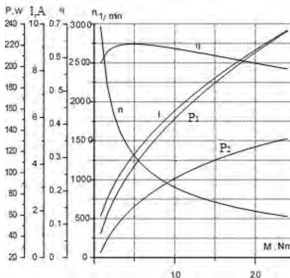
Fig. 3. SRM operational characteristics for the motor-wheel drive of the invalid chair.
