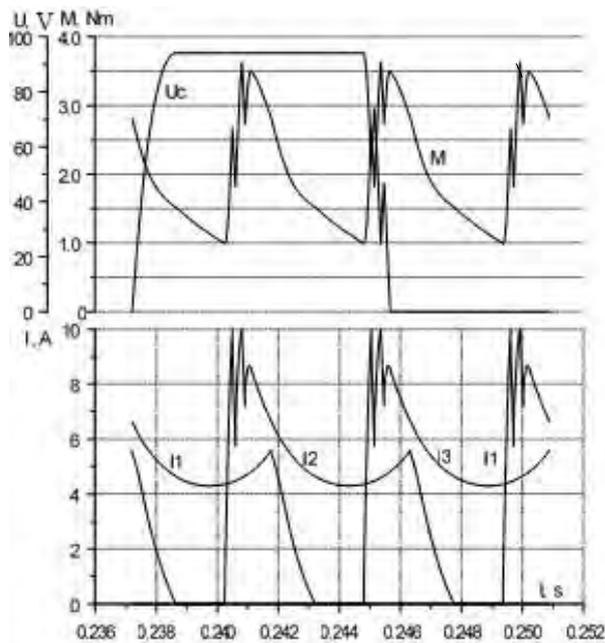
Fig. 5. Graphic presentation of currents, electromagnetic torque and voltage on the capacitor at a stable operational mode.
