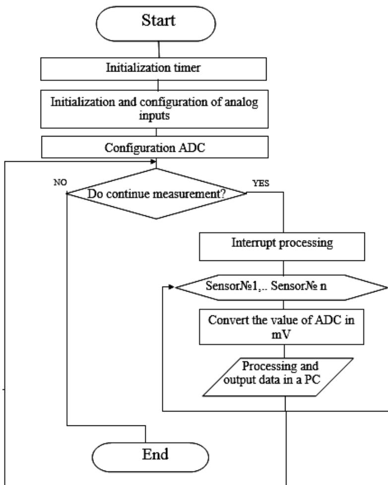
Fig. 3 Block diagram of the algorithm of the GA
