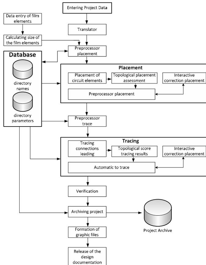
Fig. 6. Architecture CAD design engineering
