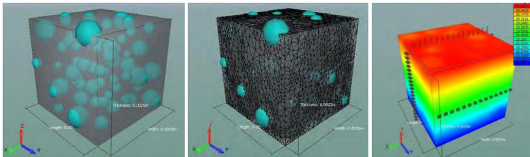
Fig.3. Example of calculating the effective thermal conductivity for composite with spherical inclusions
