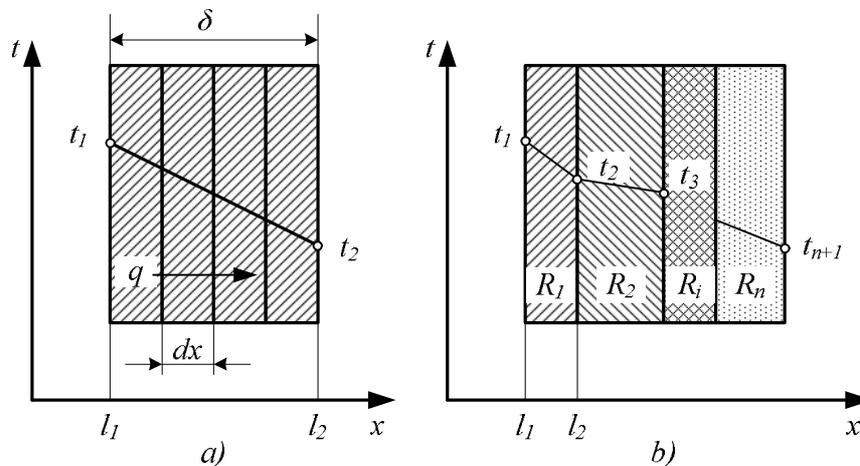
Fig. 1. Model of composite material: a – homogeneous layer; b – multilayered CM
