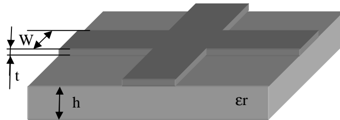
Fig. 1. The microstrip X-junction geometry and parameters list
