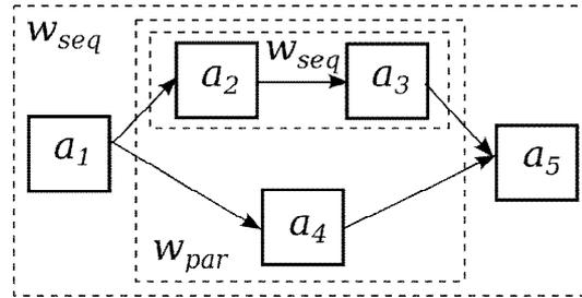
Fig. 1. Workflow example as the combination of sequential and concurrent branches
