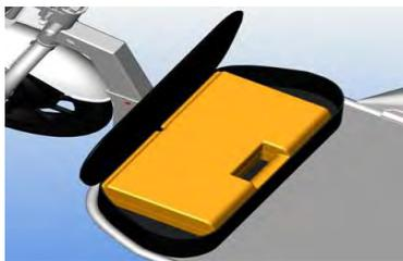
*Fig. 5. Innovation solution of a additional box for a second battery*
