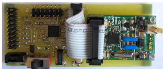
Fig.4 Photo of PLC network node
