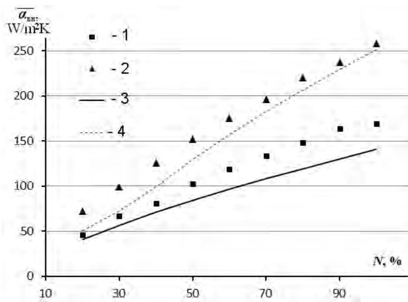
Fig. 2. The dependence of the average heat transfer coefficient  $\bar{\alpha}_{\text{BH}}$  on the surface of the pylon, which is cooled by the boiler load  $N$  at  $z = 0$  for systems of cooling airflow to the end of the pylon flat of impact jet (1), (3) and circular jets (2), (4) with different widths of pylon  $B_{\text{cm}}$ : 1,2 –  $B_{\text{cm}} = 30 \cdot 10^{-3}$  m, 3,4 –  $B_{\text{cm}} = 50 \cdot 10^{-3}$  m
