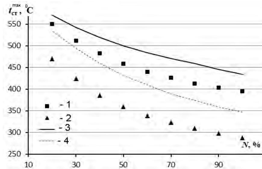
Fig. 3. The dependence of the maximum wall temperature pylon  $t_{\text{CT}}^{\text{max}}$  on the load of the boiler for cooling systems with airflow to the end of the pylon flat of impact jet (1), (3) and circuit cooling system round jets (2), (4) for different values of the width of the pylon  $B_{\text{cm}}=0,03\text{m}$  lines 1,2 i  $B_{\text{cm}}=0,05\text{m}$  lines 3,4
