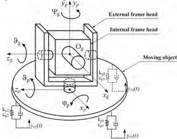
Fig. 1. General view of the searching and tracking head
