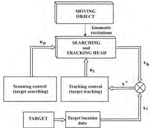
Fig.2. Control scheme of the searching and tracking head
