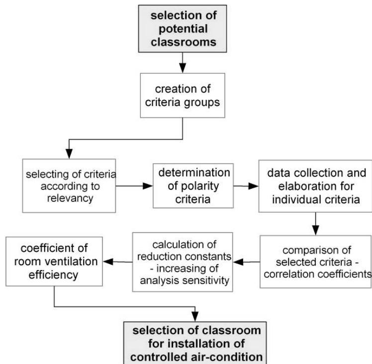
Fig. 4. Sequence diagram of multi-criteria analysis of ventilation efficiency
