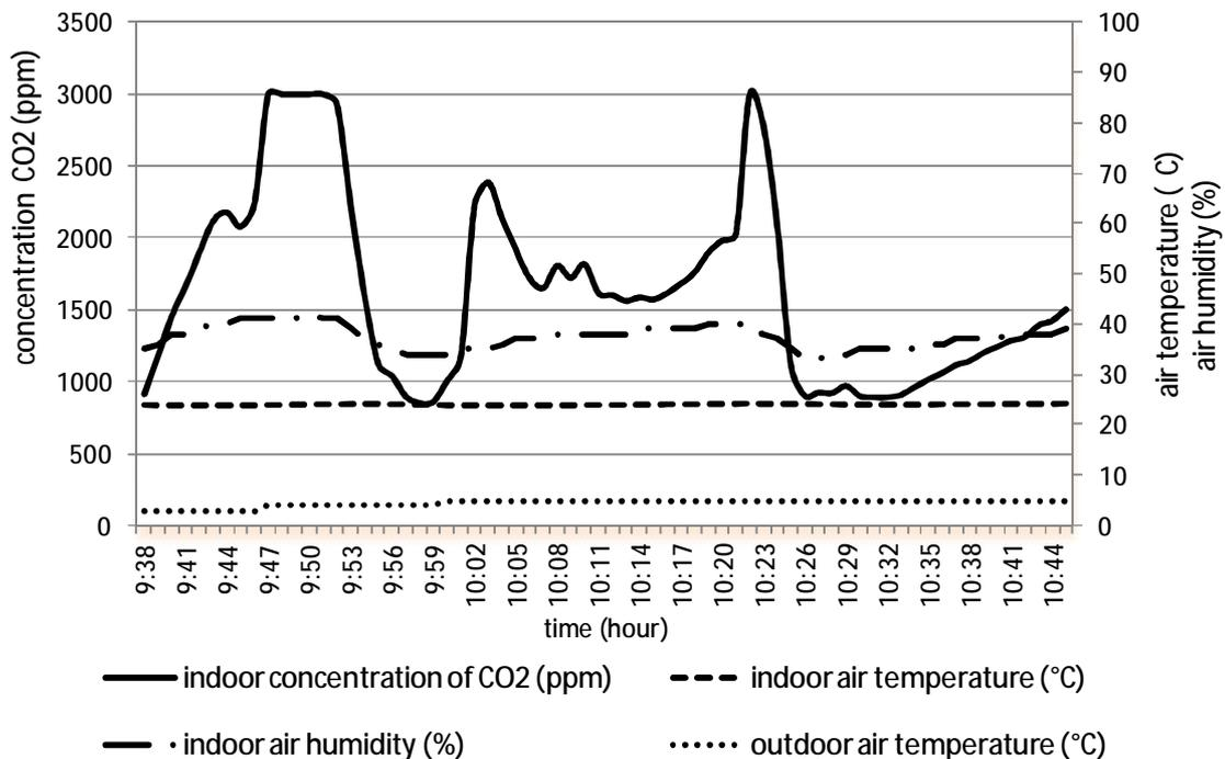
Fig. 3. Time behaviour of indoor temperatures, humidity and CO<sub>2</sub> concentration
