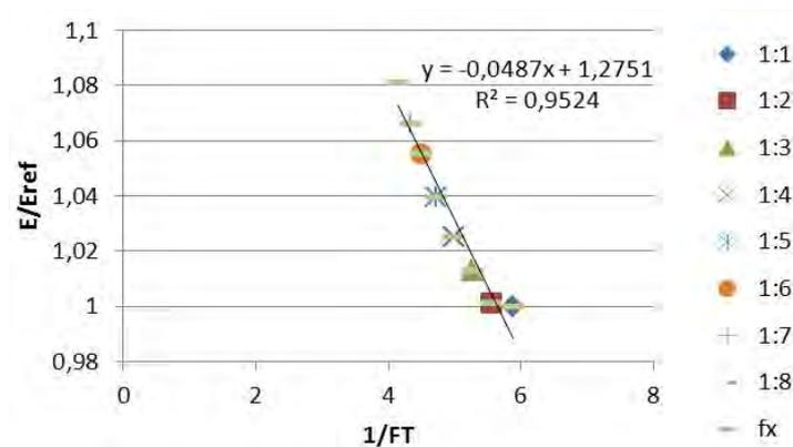
Figure 11. Linear dependence  $1/FT$  of objects with a ratio 1:1-1-8 and heating load proportionally to the heating load of reference cube the same volume
