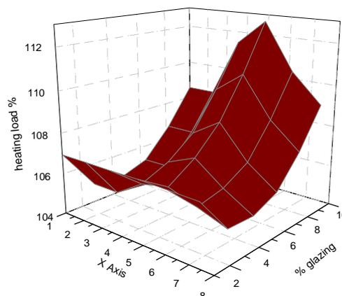
Figure 7. Heating load due to orientation and % of glazing to the external walls for shape 1 and 2
