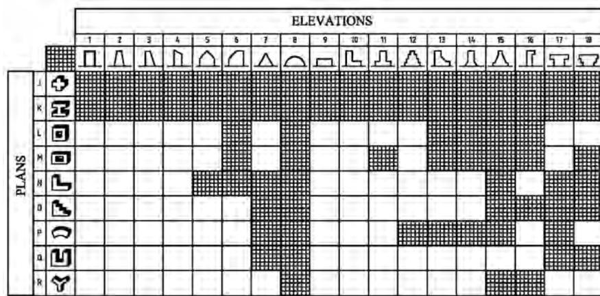
Figure 2. Created shapes of buildings – complex ground plan
