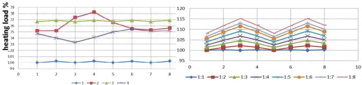
Figure 9. Impact of orientation on heating load for the shapes 1-4 (left) and 1:1-8(right)
