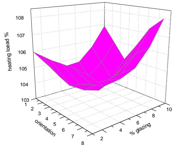
Figure 8. Heating load due to orientation and % of glazing to the external walls for shape 3 and 4
