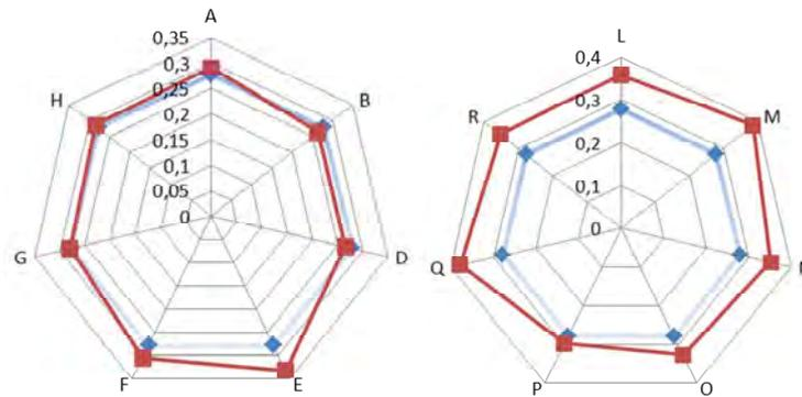
Figure 3. Shape factor: left - simple ground plan, right - complex ground plan
