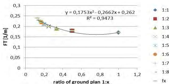
Figure 5. Effect of the ratio ground plan on shape factor on the same ground-plan area and same floor of buildings
