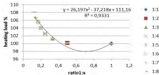
Figure 10. Regression dependency of the ratio of ground plan and heating load % (100% = cube – 1:1)
