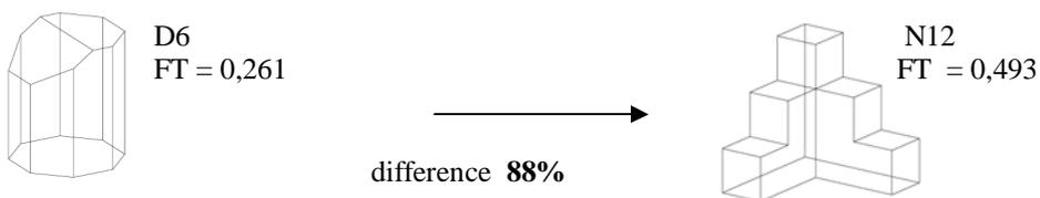
Figure 4. The difference between the maximum and minimum shape factor (FT) of the building
