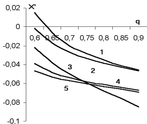
Fig. 2. Dependence of the input reactance ( $X' = X / \rho_0$ ) on  $\lambda_0$  ( $q = \lambda_0 / 2A$ ).
