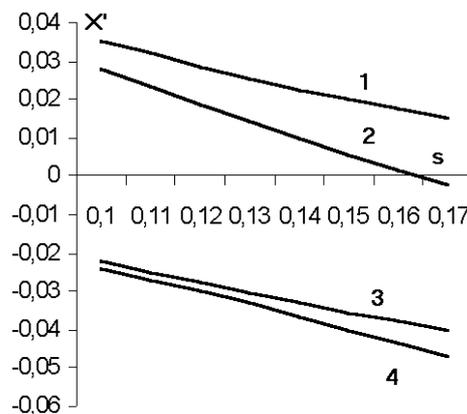
Fig. 3. Dependence of the input reactance on the vibrator's radius  $s = a / A$ .
