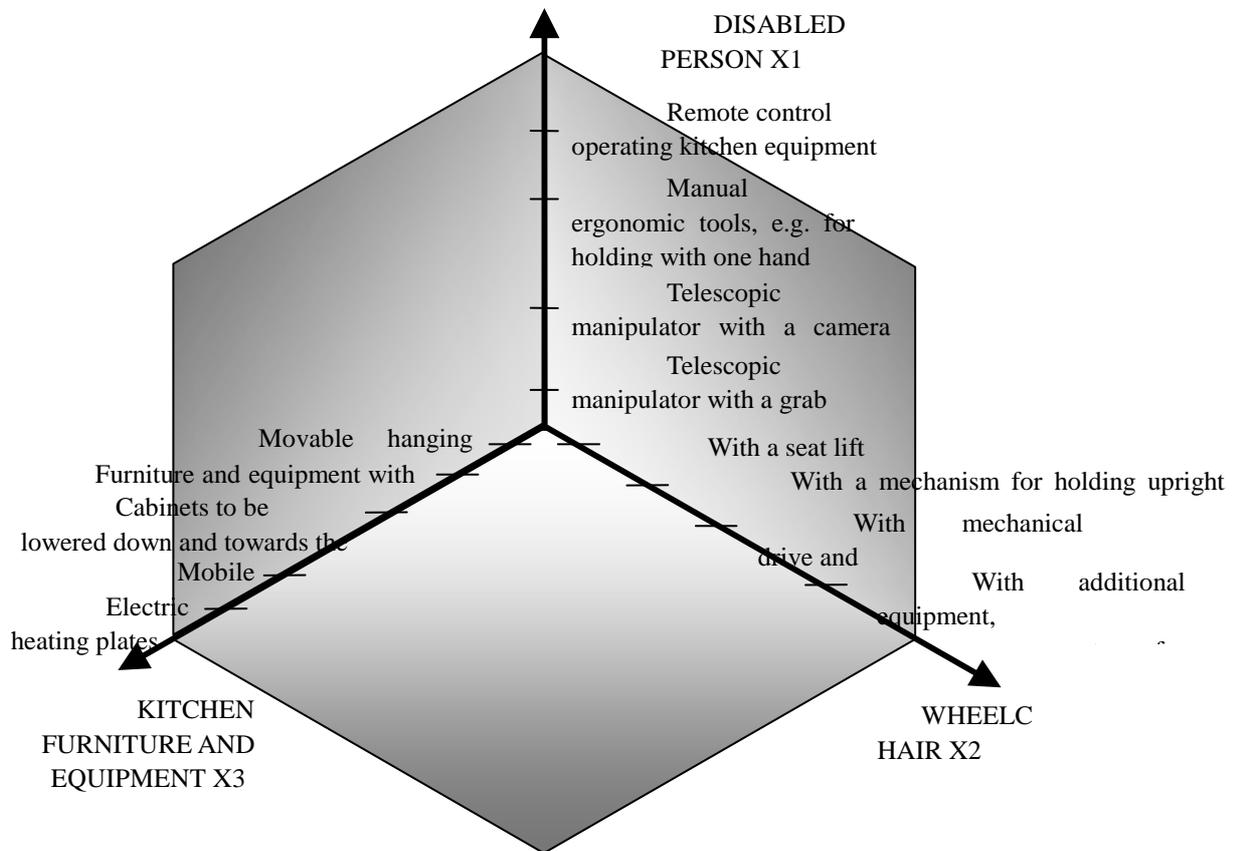
Fig. 3. Morphologic table of adaptation changes in an integrating kitchen
