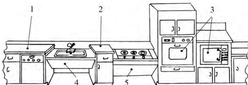
Fig. 1. An example of kitchen adaptation with row arrangement for the needs of disabled users of wheelchairs:
