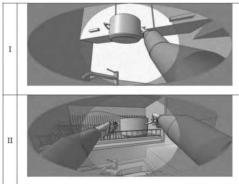
*Fig. 10. Visualisation of the field of vision of a disabled person during manipulations at the kitchen cupboard for a standard (I) and adapted (II) kitchen (Source: our own elaboration)*
