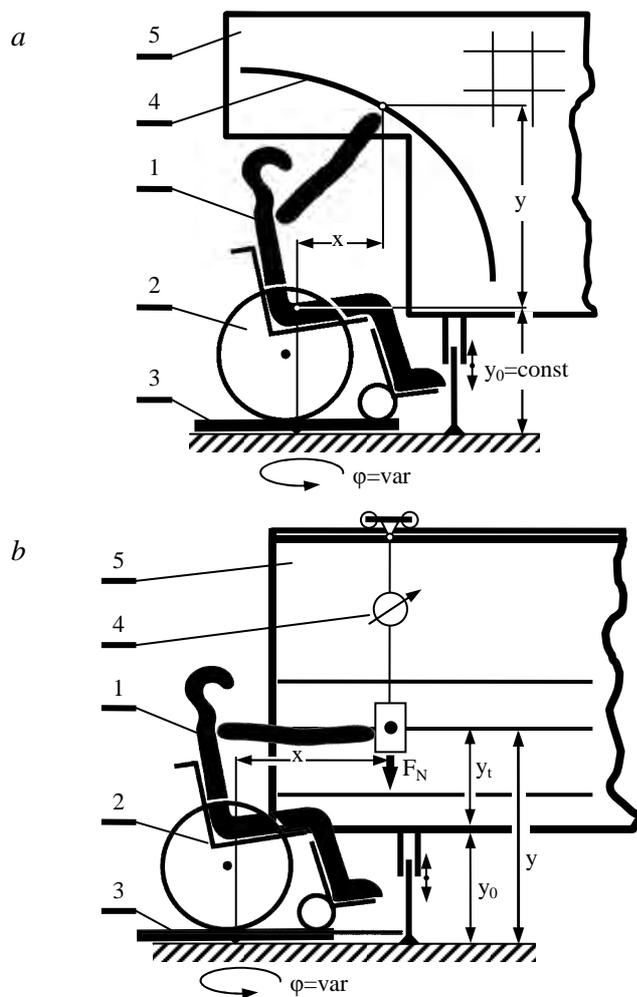
Fig. 5. Block diagram of a measurement stand and method of arm reaches (a) and arm forces (b) of a disabled person sitting on a wheelchair in a 3D space of geometrical dimensions  $x, y, \varphi$ : (1) – handicapped person; (2) – active wheelchair; (3) – measuring protractor; (4) – reach curve (a) or measuring dynamometer (b); (5) – table (Source: our own elaboration)
