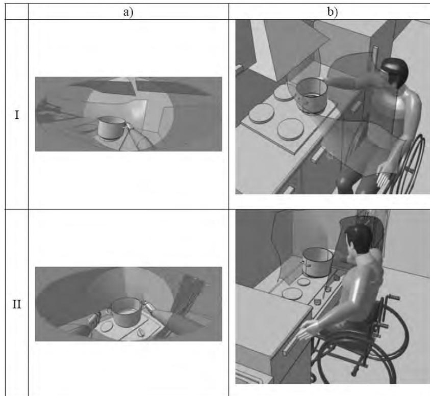
*Fig. 8. Visualisation: a) of the field of vision of a disabled person during manipulations at the gas cooker and b) manipulations possibilities of the right arm for a standard (I) and adapted (II) kitchen
