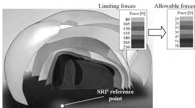
Fig. 6. Set of surfaces determining zones of occurrence of constant forces of the right arm against the external surface of the arms' reach
