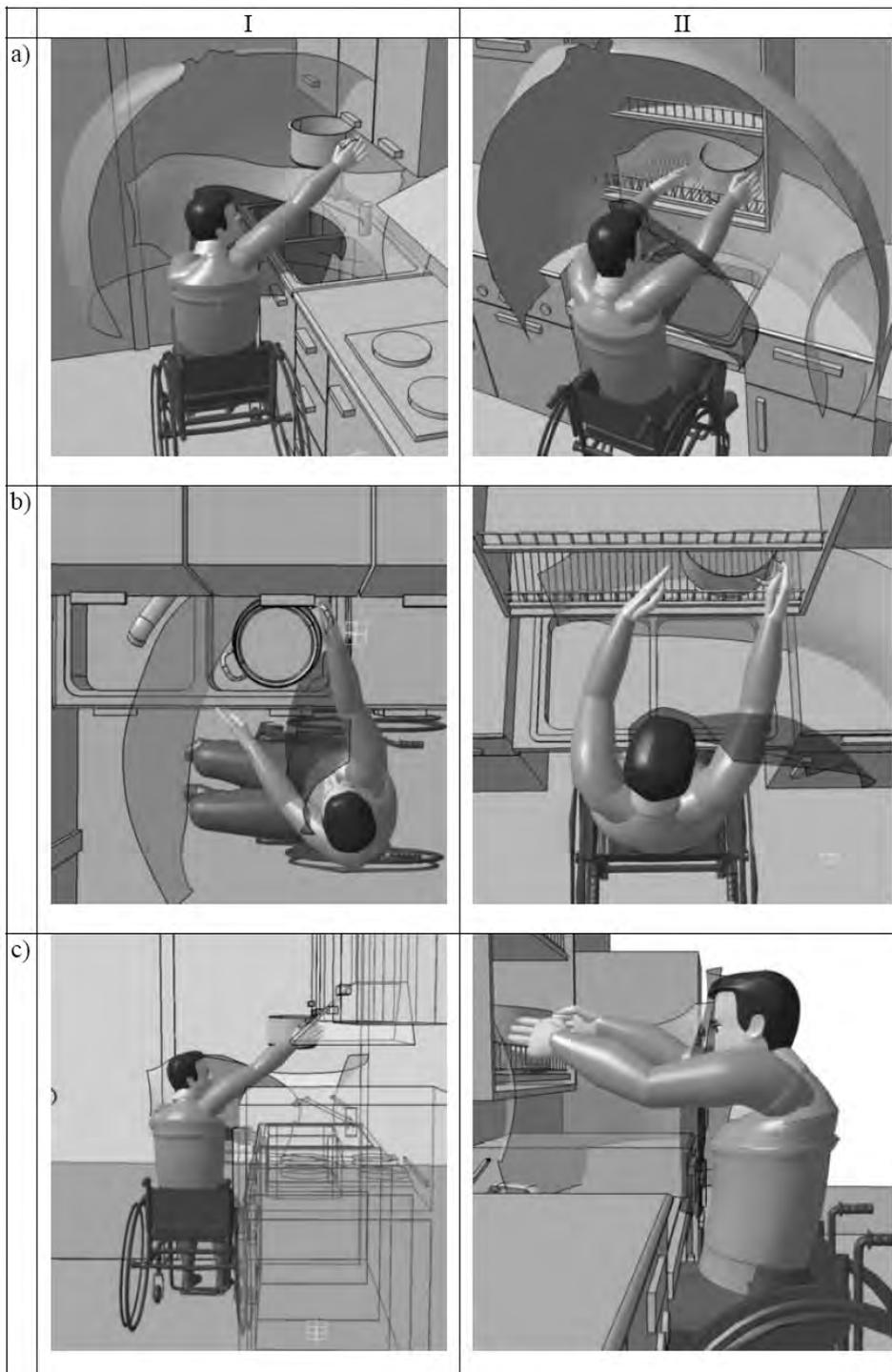
*Fig. 9. Visualisation of the area of reach of the right hand and the force range during manipulations at the upper cabinet for a standard (I) and adapted (II) kitchen; red colour – 180 N zone, beige colour – 80 N zone, grey colour – maximum range of arm reach
