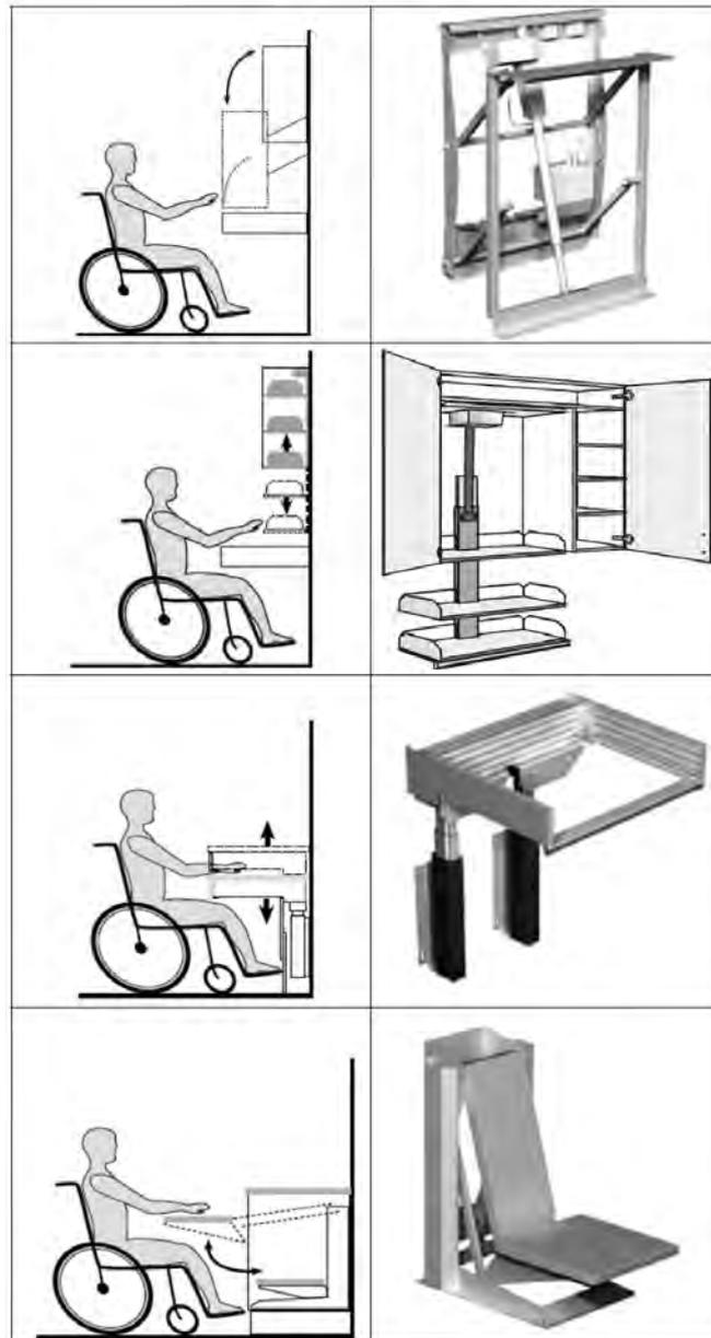
*Fig. 4. Mobile kitchen furniture in applications for the disabled and structural principles
