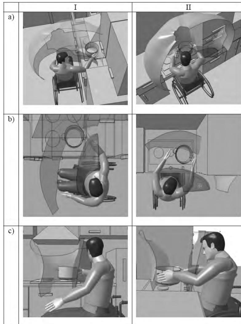
*Fig. 7. Visualisation of the reach zone of the right arm and force range during manipulation at the gas cooker in a standard (I) and adapted (II) kitchen; red colour – 180 N zone, beige colour – 80 N zone, grey colour – maximum range of arm reach (Source: our own elaboration)*
