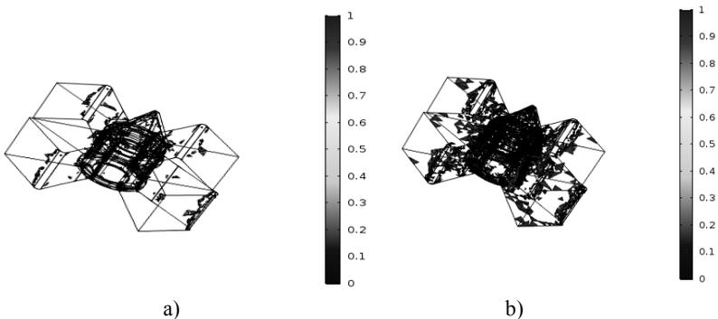
Fig. 2. The number of the worst elements (10% (a) and 25% (b) from the total amount) of the 3D mesh of the element model of the surge protection system.
