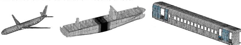
Fig.1 Typical Finite Element Models of Structures Constrictions
