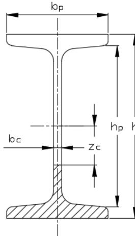
Fig. 2 I-beam cross section
